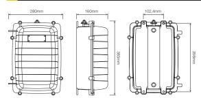
Tunnel Ray is versatile and can be backed with optional Coolon Emergency Pack. Emergency Tunnel Ray can be wired to be both maintained and non-maintained, eliminating the need for costly additional fittings. The Emergency Tunnel Ray will work for a minimum of 2 hours in case of power failure, far exceeding the requirements of Australian Standards.
