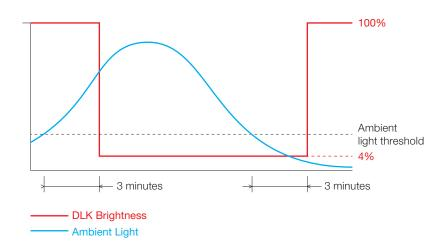
The DLK LED will be at 100% brightness when it is turned on and then will dim to 4% brightness when daylight is detected. 3 minutes after the daylight has dropped below the minimum ambient light threshold, the DLK LED will ramp up to 100% brightness. (Only applies to DLK equipped with light sensor)
