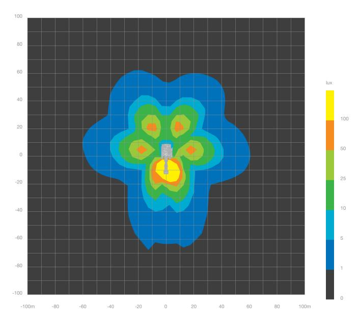
Light loss/maintenance factor: 0.85 Ambient temperature: 35°C
