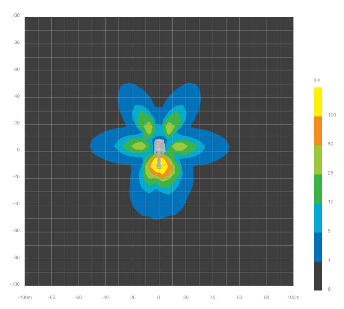
Light loss/maintenance factor: 0.85 Ambient temperature: 35°C
