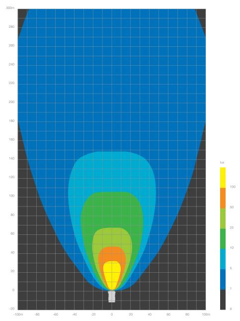
Light loss/maintenance factor: 0.85 Ambient temperature: 35°C
