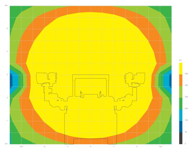
Light loss/maintenance factor: 0.85 Ambient temperature: 35°C
