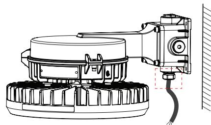
**WARNING** - Cable entry points not in use need a plug installed.
