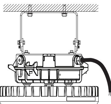
**WARNING** - Cable entry points not in use require a plug installed.
