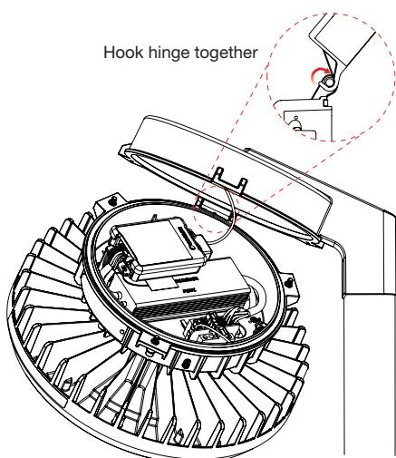
**WARNING** - Cable entry points not in use require a plug installed.
