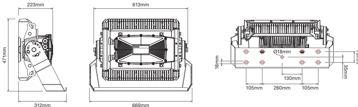
**STELLAR Luminaires with Dragline Mounting Bracket**
