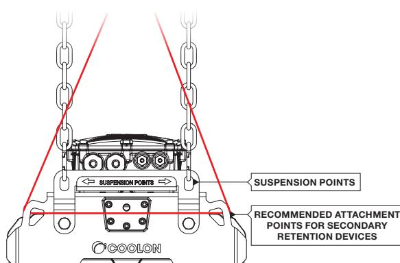
The lanyard attachment points allow for a luminaire drop not exceeding 200mm under normal conditions.
