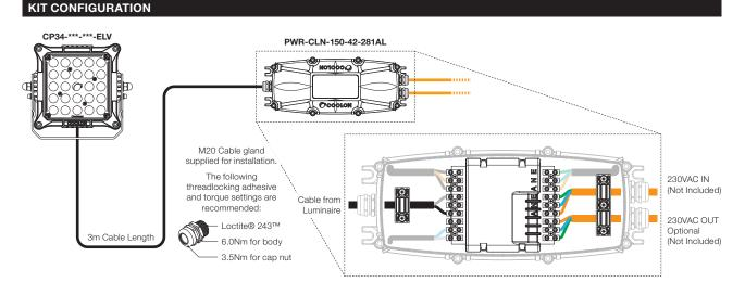
Distance between the power supply and luminaire can be extended up to 15m. The voltage drop on the cable must not exceed 2V. A wiring connection must be made from the input wiring terminal to the loop out terminal where optional loop out is required.
