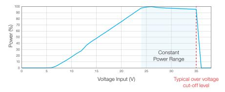
The CP24 is designed to be connected to a low impedance 24VDC source such as a battery or a suitable Power Supply directly using up to 2 metre cable.
