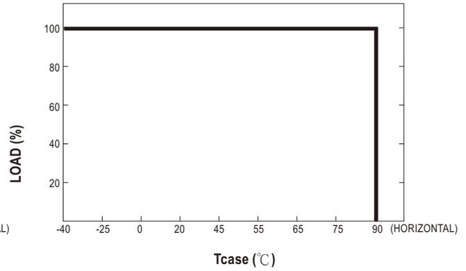
© If HLG-480H operates in constant current mode with the rated current, the maximum workable  $T_a$  is 60°C. (Typ. 230VAC)
