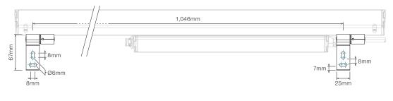
$\begin{array}{l} \mbox{\bf MINIMUM RECOMMENDED FASTENERS PER LUMINAIRE:} \\ 4 \ x \ M5 \ bolts \ for \ single \ luminaires \end{array}$
