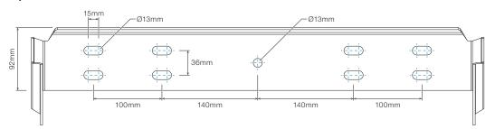
MINIMUM RECOMMENDED FASTENERS PER LUMINAIRE: 4 x M12 bolts for double and triple luminaires
