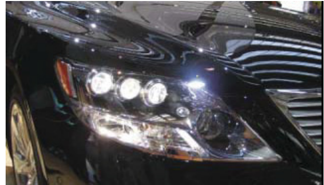
Fig. 4. The Lexus LS600h uses LEDs for the low-beam function only.
