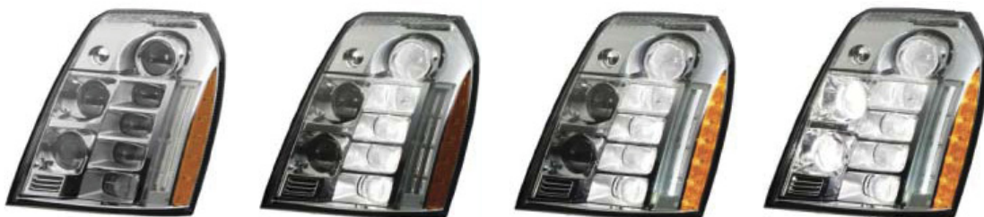
Fig. 2. LED headlamps for the Platinum Escalade, shown with (a) LEDs off, (b) daytime running light on, (c) low beam headlamps on, with position light and side marker, and (d) main beam headlamps on. The headlamps from Hella use LEDs from Osram Opto Semiconductors.
