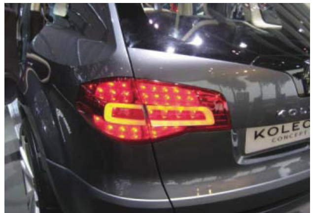
The Koleo concept car from Renault made full use of LEDs for rear lighting (above) and forward lighting (below). Also visible is the unique wing mirror containing a white LED position light and a dual amber light-guide for the indicator.
