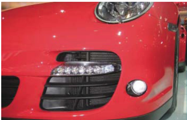
Porsche was one of a number of manufacturers, including Audi, Aston Martin and VW, to use white LEDs for daytime running lights (DRLs) on production vehicles (but still mainly high-end models).
