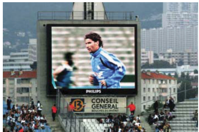
Fig. 2. C-nario supplied a content-based network for Olympic de Marseilles's Stade Velodrome that includes 2 Philips LED screens measuring 56 m 2 each, with 25 mm pitch and 256 x 352 resolution
