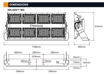
Optional Beam Coupling Plate for XBLADE™ 960 ACC-BCP-BC400-PL330-MS (available separately)
