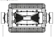
50x50x5mm angle bracket on existing frame of dragline. User must prepare the frame for installation.
