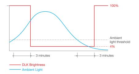
The DLK LED will be at 100% brightness when it is turned on and then will dim to 4% brightness when daylight is detected. 3 minutes after the daylight has dropped below the minimum ambient light threshold, the DLK LED will ramp up to 100% brightness. (Only applies to DLK equipped with light sensor)
