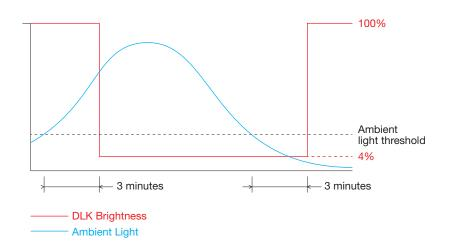
The DLK LED will be at 100% brightness when it is turned on and then will dim to 4% brightness when daylight is detected. 3 minutes after the daylight has dropped below the minimum ambient light threshold, the DLK LED will ramp up to 100% brightness. (Only applies to DLK equipped with light sensor)
